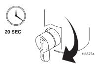
12. Raise siphon tube above flushing fluid and run sprayer for 15 to 30 seconds to drain fluid. Turn pump switch OFF. Turn engine **OFF**.
