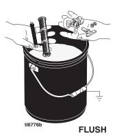
6. Remove siphon tube set from paint and place in flushing fluid. Use water for water base paint and mineral spirits for oil base paint.
